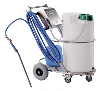
**SCHAUMHEXE 100 L** – mobile facility with lance and accessories. The Schaumhexe draws in chemical concentrate via a pneumatic pump and adds it in a selectable ratio to the water from the storage tank (100 l). It is also possible to supply a ready-mixed dilution of chemical agent and water. VA mobile cart; 12 m foam hose; 10 m air hose 6 mm; minimum air pressure: 8 bar.
